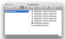
Copy the top level Reel folder (A002R20Z in the above example) to another storage device to back-up the image data. Any copy tool can be used to back-up files from the Capture Drive to another storage device.
