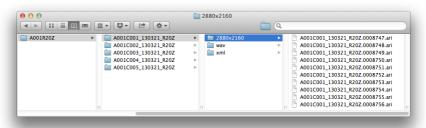
Copy the top level Reel folder (A001R20Z in the above example) to another storage device to back-up the image data.
