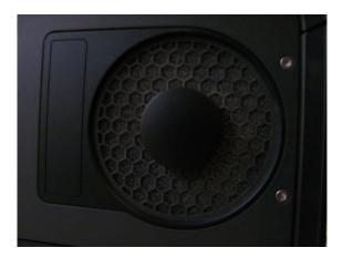
Remove the air intake grill. It is clipped in place but can be freed with a small amount of movement to the left and right whilst pulling gently. A pair of needlenose pliers can be used for this, holding the grill near to the central disk:
