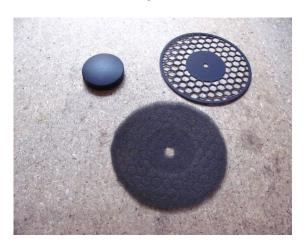
Then refit the filter material. When refitting the air intake grill, note the locating pin. This should be at the top of the grill when refitted:
